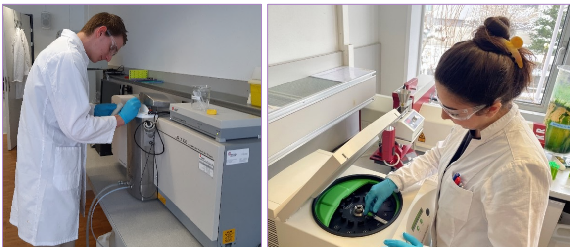
Figure 16 Measurement of a PSD at the HSLU: left laser diffraction, right optical centrifuge.
